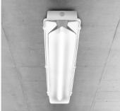
Catalog #: GLT4-S-L80-UNV-DM-C50-CA Photometric Test Report #: 10542601-795084 Delivered Lumens: 8369 Efficacy (Lumens/Watt): 115.9 Power: 72.16w @ 120 VAC Power Factor: 0.995 Current THD: 7.74% CRI: 83.7 CCT: 5047 K LED Life: 50,000+ hrs
