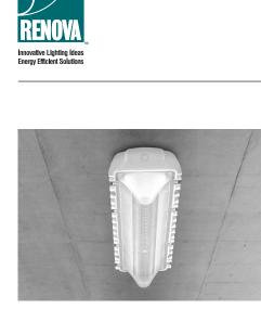
Catalog #: L-WDG2-MN-L35-UNV-37DM-W36-C40-FA Photometric Test Report #: 10405943-691886 Delivered Lumens: 3541 Efficacy (Lumens/Watt): 97.8 Power: 36.20w @ 120 VAC Power Factor: 0.994 Current THD: 5.88% CRI: 84.8 CCT: 4237 K LED Life: 50,000+ hrs
