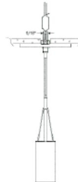
T2 - 9/16" Bolt Slot T-Bar Mount
